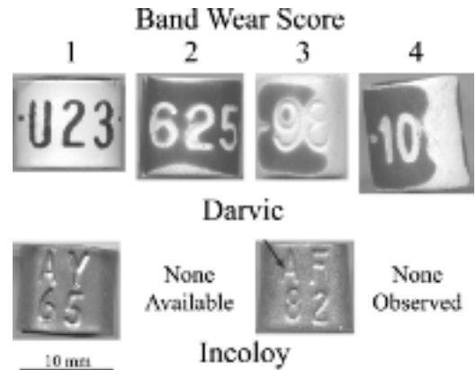
Fig. 1. Worn darvic and incoloy bands representing band wear scores 1–4: no wear, (1); all characters easily read, (2); one or more characters difficult to read, (3); one or more characters illegible, (4). The arrow identifies a character on an incoloy band that may fit the criterion of “difficult to read” in the field. Score 2 and 4 on incoloy bands were not available and not observed, respectively.
